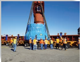
Off-loading the 107mt hub end forging from the inter-marine ship onto an eight-axle line dual lane heavy haul trailer; this is the beginning of the multi-day trip from Long Beach pier-F to the job site in Las Vegas
