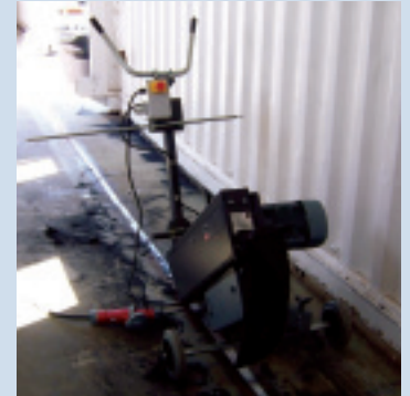
A STAND UP grinder is used to grind the deck weld
