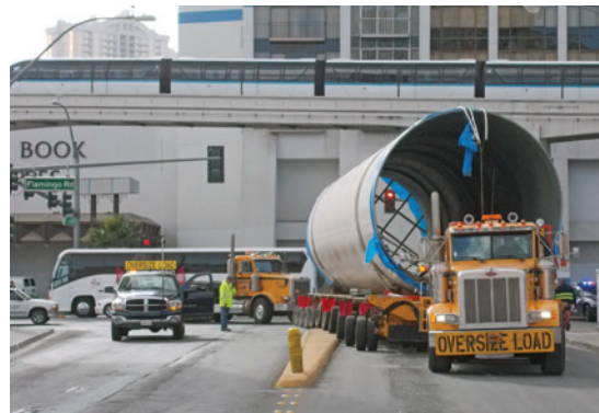
At over 14' diameter, 77' long and 116-ton in weight, the hub mid-section arrives in Las Vegas from Port of Long Beach
